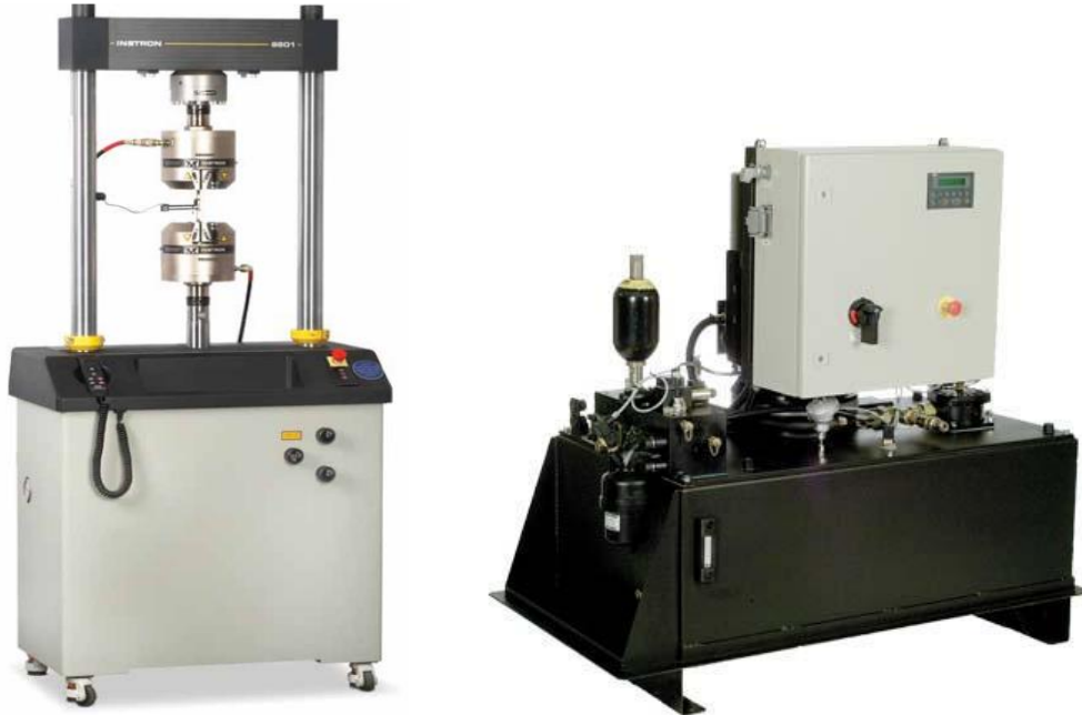
Figure 26: (a) Instron 8801 compression and fatigue testing machine used in the study (b) Instron 3580 Hydraulic power unit
