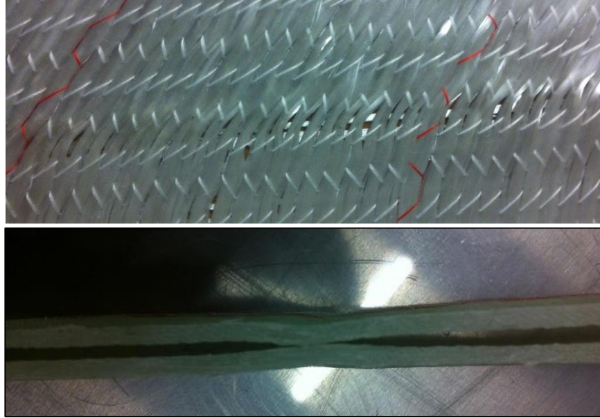
Figure 9: (a) Tow thinning seen in a fabric on shifting 35° (b) Out of plane defects identification visual inspection for 25° Shifted fabric.
