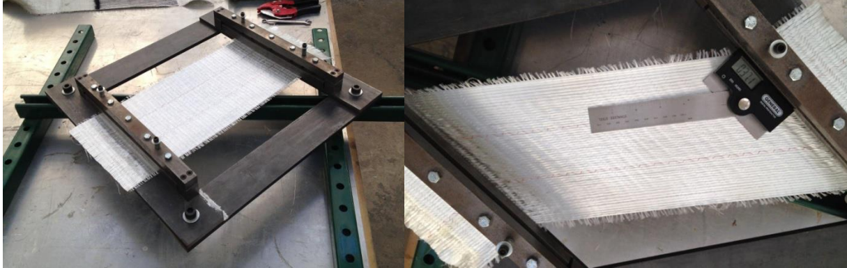
Figure 21: [a] Shear lock limit testing setup; [b] The shear lock limit measuring on anunidirectional fabric
